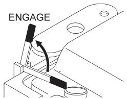
Figure 39. Transmission Engage/Disengage Lever (Engage Position)
